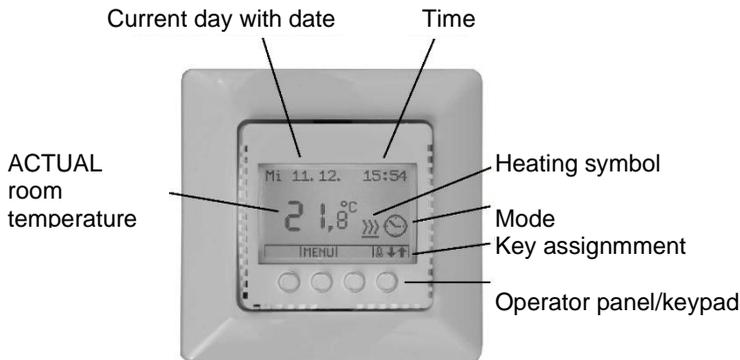
**Turning on the controller for the first time:**
